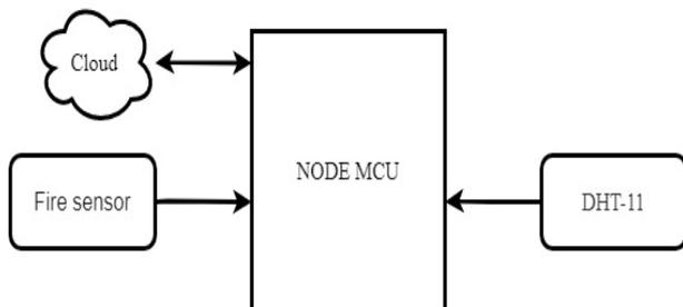
Figure 1: Block diagram of a Fire detection system
