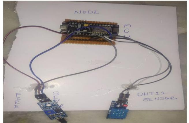
Figure 3: Fire detection system experimental setup
