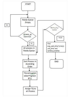
Figure 5: Flowchart of Improvised version of Round Robin Algorithm
