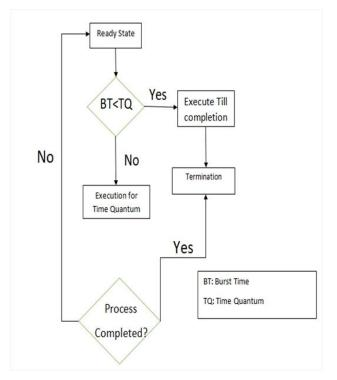
Figure 3: Flowchart of working of Round Robin Algorithm
