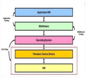
Figure 1: Operating System Framework
