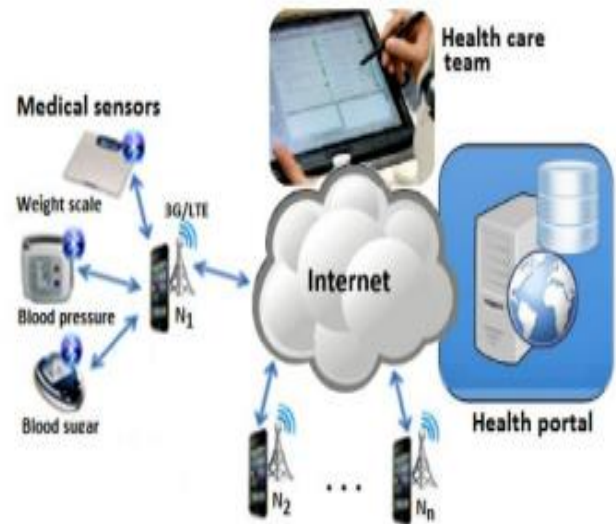
Figure 4: Illustrate the diagram Architecture of the smart phone based e-Health System
