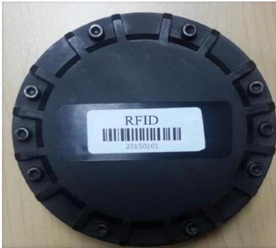
Figure 3: Manhole's cover with RFID
