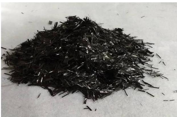
Figure 1: Sample of carbon fiber
