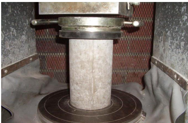
Figure.3: shows the loading on Concrete specimen
