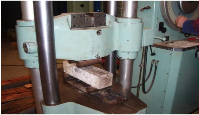
Figure 4: The flexural strength test
