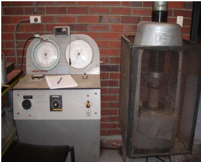
Figure 2: the image of compressive testing machine
