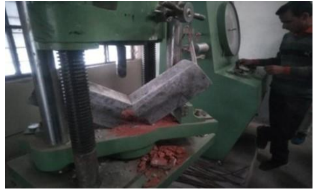
Figure 9: Flexural strength test of concrete
