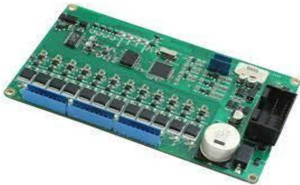
Figure 4: Block BMS Board
