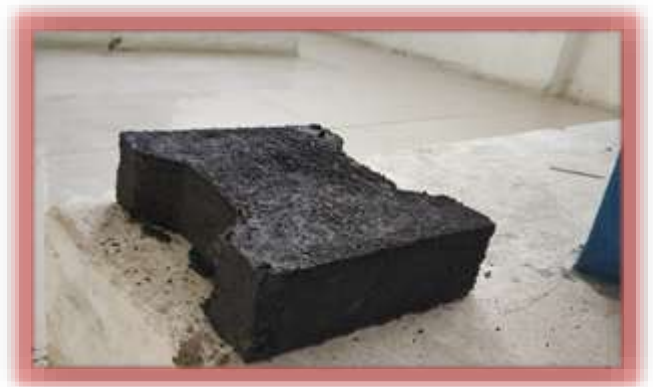
Figure 2: Moulded Shape of Brick and Paver Block After 24 Hours
