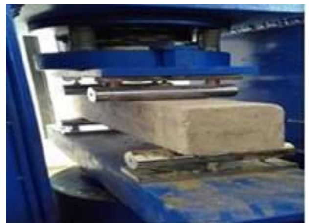
Figure 7: Flexural Strength Test
