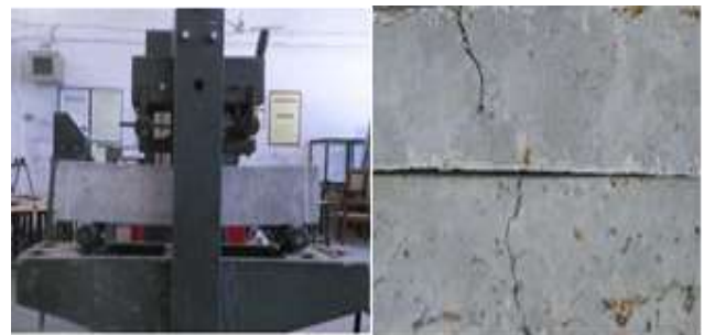
Figure 10: Flexural crack, Figure 11. Three point loading machine
