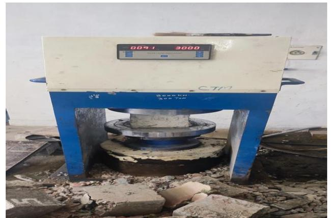
Figure 2: Sample on Compression Testing Machine
