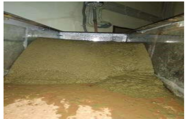
Figure 2: Slope failure and soil erosion at high intensity (i=1.2mm/hr) with using jute mats
