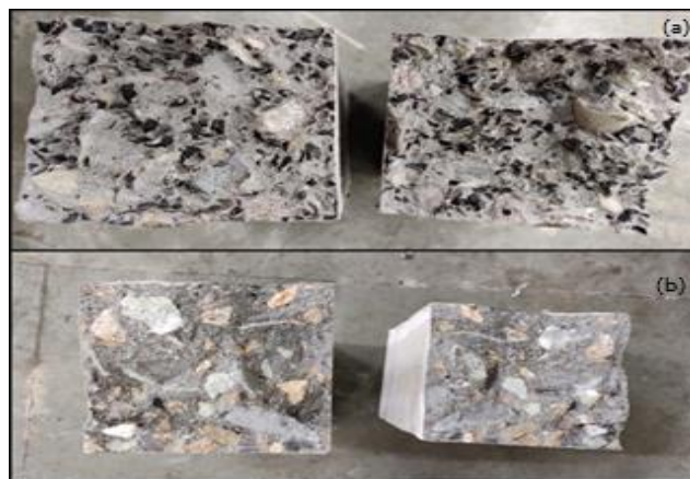
Figure 1: Representation of SCM induced Rubcrete Beam (a) and Plain cement Concrete Beam (b)
