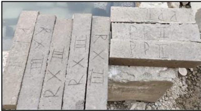
Figure 4: Flexure beams to be put in curing tank
