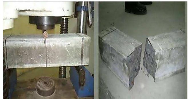
Figure 13: Flexural Testing Set up
