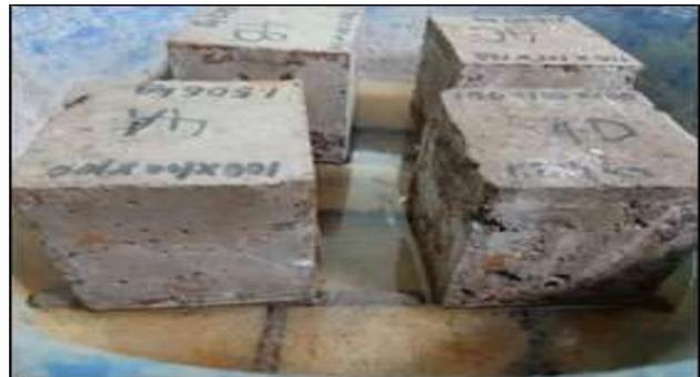
Figure 6: Setup of experiment for porosity test
