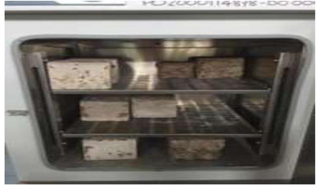
Figure 5: Soil sample placed in the oven
