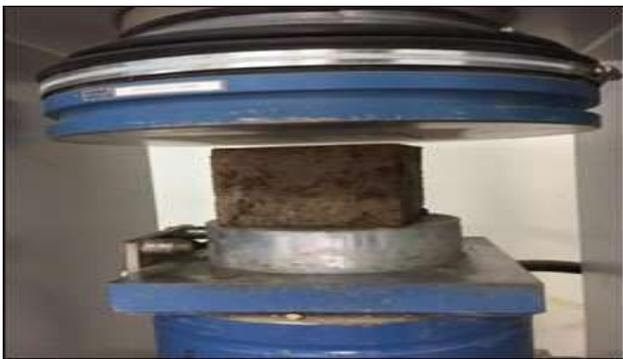
Figure 7: Compression test for the soil sample
