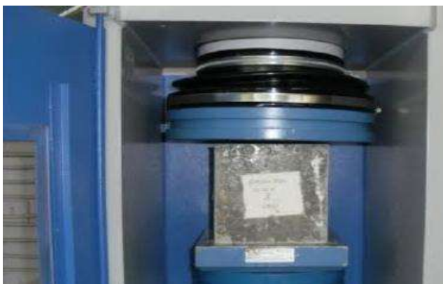
Figure 1: Compressive Strength Test on Cubes
