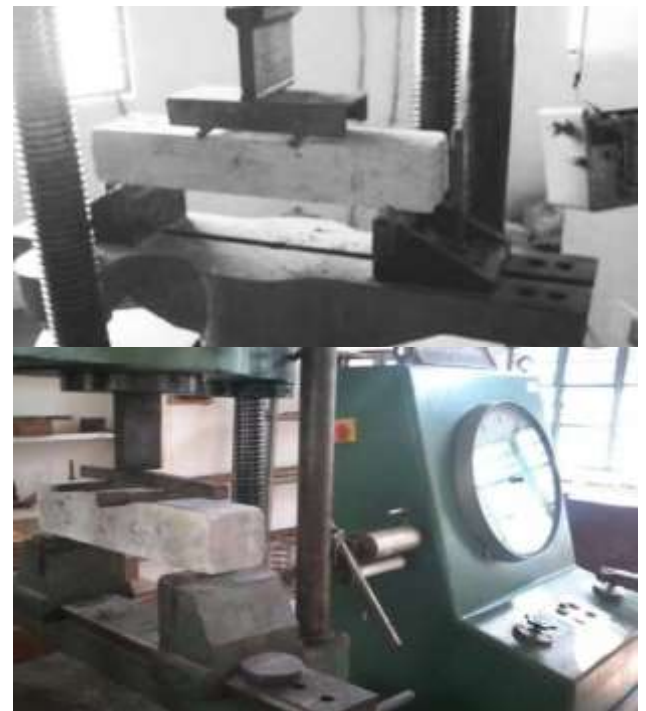
Figure 2: Flexural Strength Test on Beams
