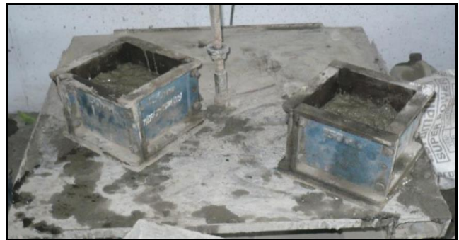
Figure 1: casting of cubes
