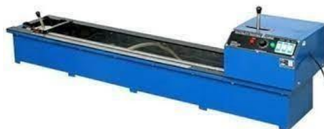
Figure 3: Ductility test apparatus
