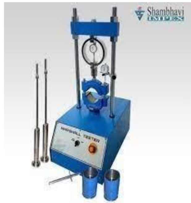
Figure 5: Marshall stability test apparatus
